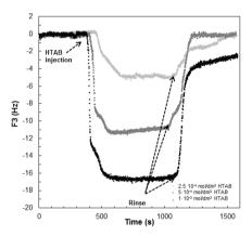
Fig. 1. Displays the real-time experimental data of the frequency  $\Delta f3$  from the third overtone associated with HTAB adsorption onto quartz surface for different HTAB concentrations at natural pH (6.5)
