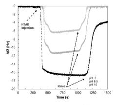
Fig. 2. Real-time experimental data of frequency shifts for different pH (3, 5.5, and 10) at constant HTAB amount  $(5 \cdot 10^{-4} \text{ mol/dm}^3)$
